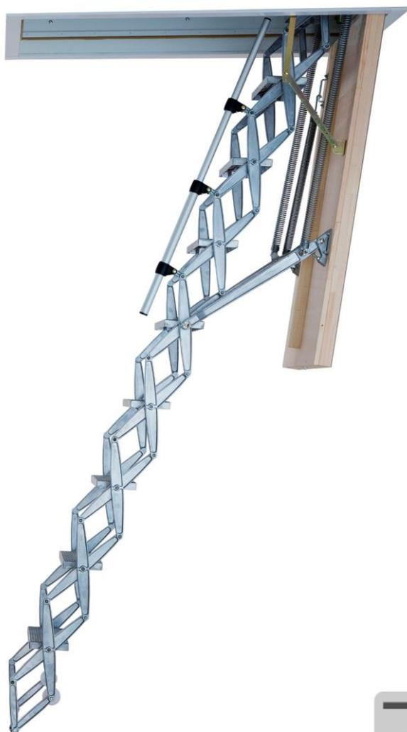
The Supreme heavy duty aluminium loft ladder is manufactured from quality die-cast aluminium alloy components for strength and light-weight operation. The wooden hatch box and insulated trapdoor provide excellent energy efficiency.
